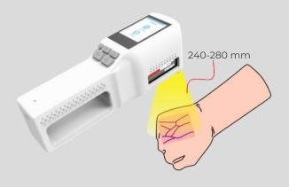
Generates a projection of subcutaneous vein blood vessels using infrared light.
